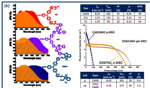
(b) Overlaid IPCE plots for a P1, GS1, CAD 3 NiO p-DSC and a D35 TiO<sub>2</sub> n-DSC (orange), as well as current-voltage plots for the record cells.
