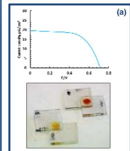
(a) Tandem QDSSC utilising CdSe on NiO and CdSe<sub>0.85</sub>S<sub>0.15</sub> on TiO<sub>2</sub>
