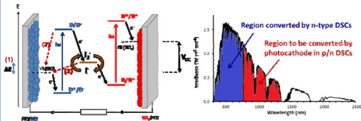
Figure 1: Schematic of tandem cell structure
